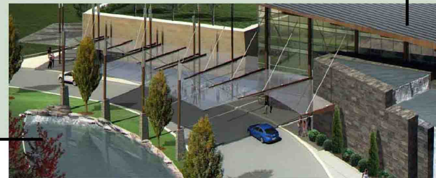
Roof overhangs to shade and cool the building face
