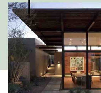
Roof overhangs to shade and cool the building face
